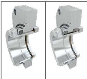
Single and Double O-ring Seal Traditional general purpose seal. Low cost and easy to service. Suitable for low pressure applications. 100 psi, 7 bar
