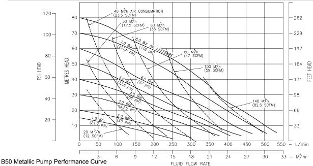
Performance based on water at ambient temperature
