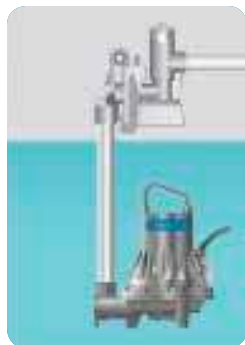
H-INSTALLATION Stationary wet installation suspended from the discharge pipe. The quick connection joint has an integrated non-return valve applicable to Flygt Compit pump station.
